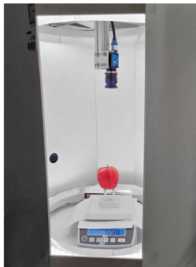
Machine vision system for taking 2D images of apples
